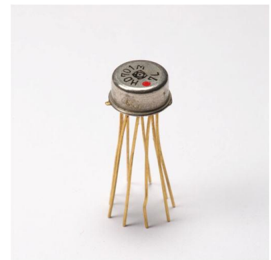
MOS IC for calculator 10-pin TO-5 package
