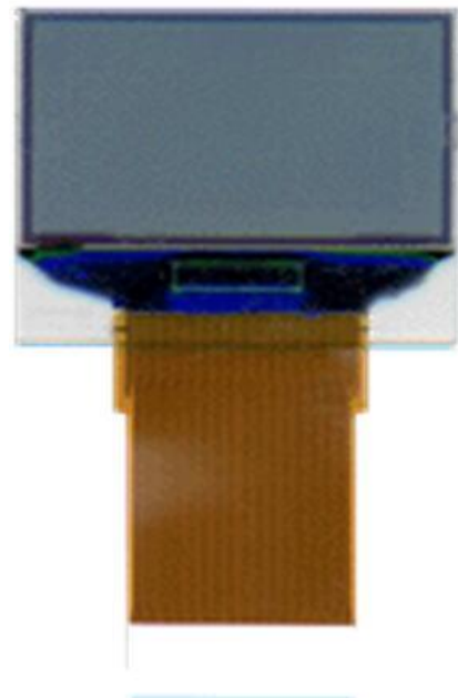
Fig.2: Example of COG Assembly (By courtesy of Hitachi)
