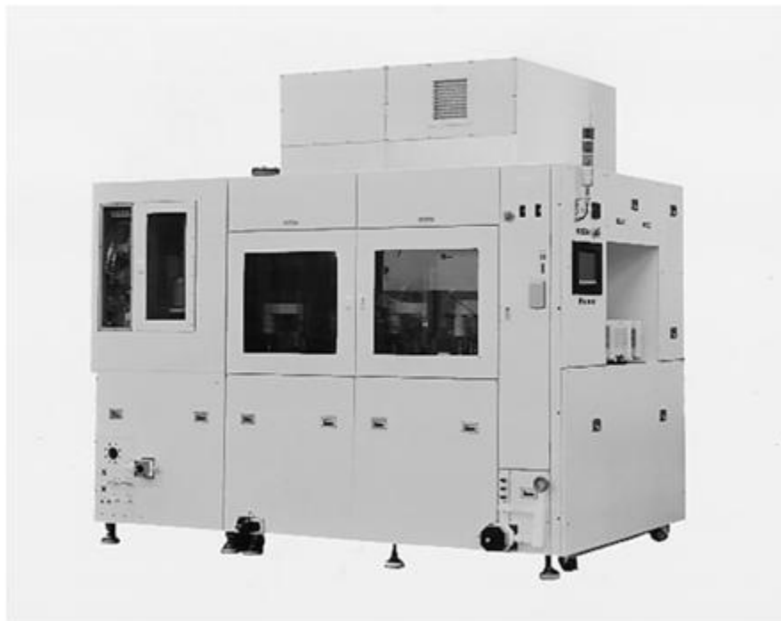
Fig.2: Early dry-in/dry-out CMP equipment EPO-1141 (By courtesy of Ebara Seisakusho)
