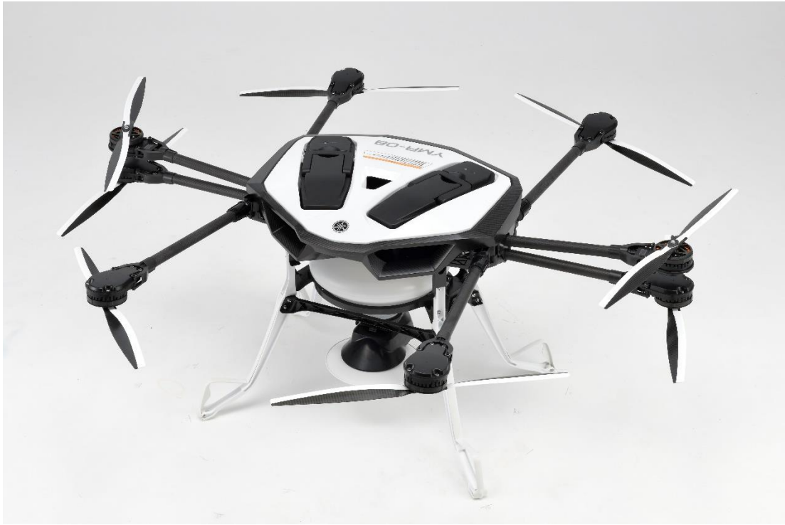
Figure 2 Industrial-use multirotor YMR-08 (Model L80) (1,923mm(L)×2,181mm(W)×669mm(H), Number of rotors: 8, Rotor diameter: 26inch(66mm)) (Rated battery capacity: 852 Wh) (Motor torque: (maximum) 2.4 Nm/4,000 rpm, (continuous output) 1.2 Nm/2,800 rpm) Courtesy of Yamaha Motor Co. Ltd.
