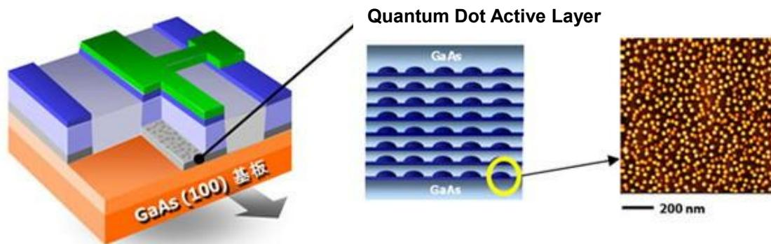
Schematic of quantum dot laser structure
