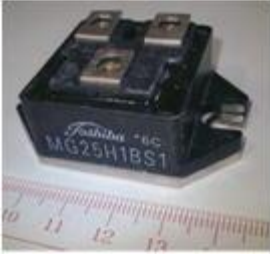
Photo 1: Non-latch up type IGBT first released by Toshiba (By courtesy of Toshiba)
