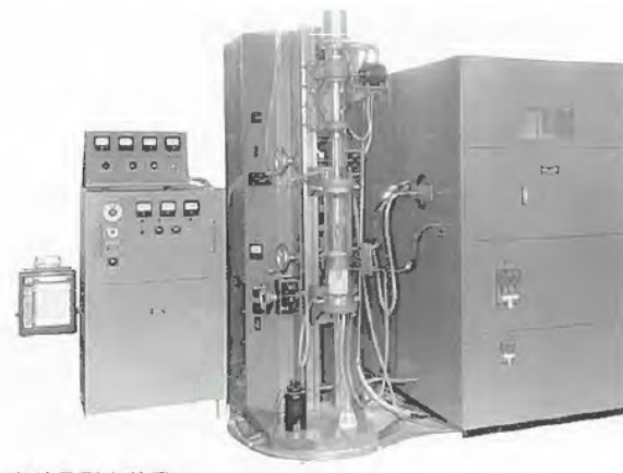
Figure 1 Germanium/silicon single crystal pulling equipment (provided by KOKUSAI ELECTRIC)
