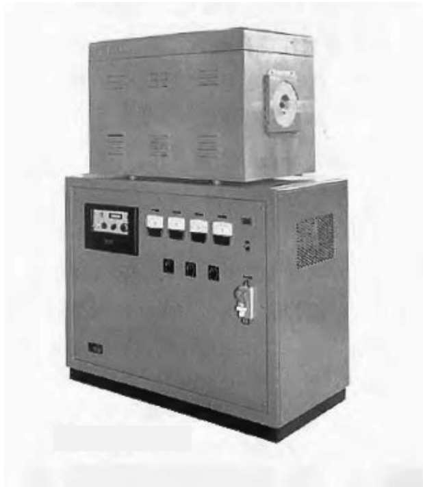
Figure 1 Horizontal Diffusion Furnace (DD-1) (provided by Kokusai Electric Corporation)
