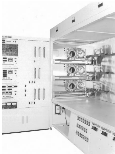
Figure 1 LPCVD Equipment (DJ-8300) (provided by KOKUSAI ELECTRIC Corporation)
