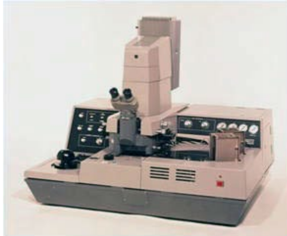
Figure 1 The first Proximity Aligner (PPC-1) (provided by Cannon Inc.)
