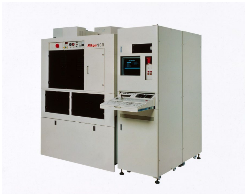
Figure 1 i-line stepper (NSR-1755i7) (Courtesy of NIKON CORPORATION)
