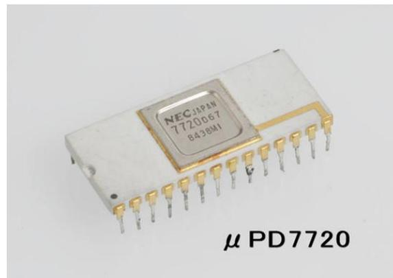
Fig. One-chip Digital Signal Processor  $\mu$ PD7720
