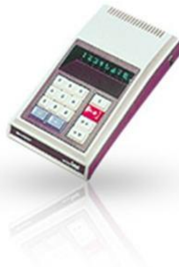
Figure: World first LSI Calculator QT-8D(Sharp)
