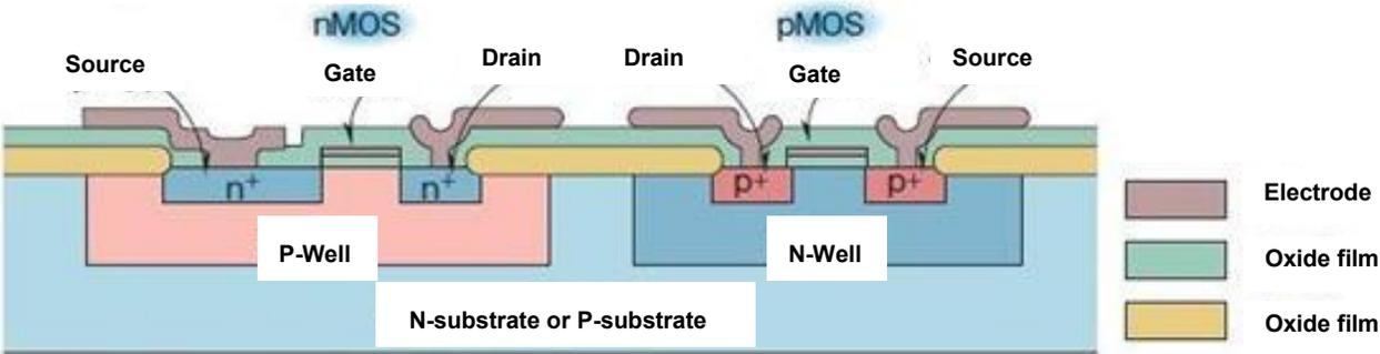
**Devised twin-well CMOS technology realizing high-speed performance**
