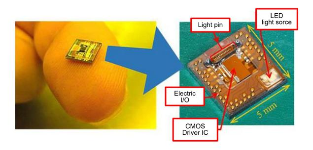
Fig.1 Light transceiver of 5mm□ by silicon photonics (By courtesy of NEDO/PETRA)
