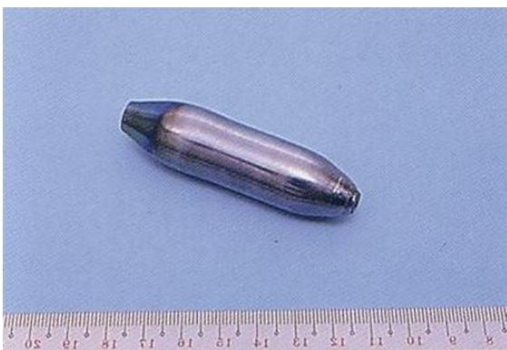
Silicon single crystal ingot pulled by Toshiba in 1956
