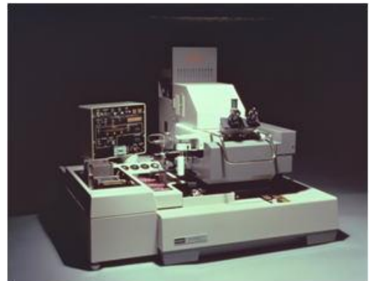
Proximity Exposure Equipment with Automatic Alignment PLA-501FA (By courtesy of Canon)
