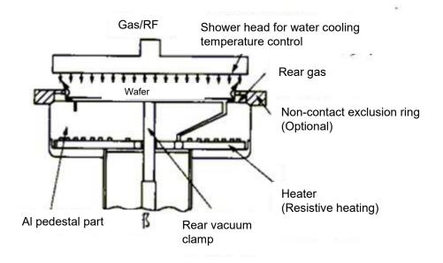
Fig.2: Structure example of plasma CVD equipment (Chamber part)
