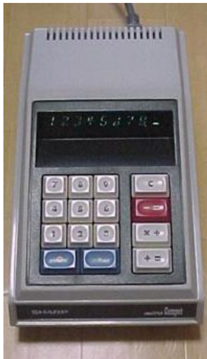
Photo 2.3 World’s first LSI calculator QT-8D developed by Sharp (1969) 4 LSIs were manufactured by North American Rockwell.
